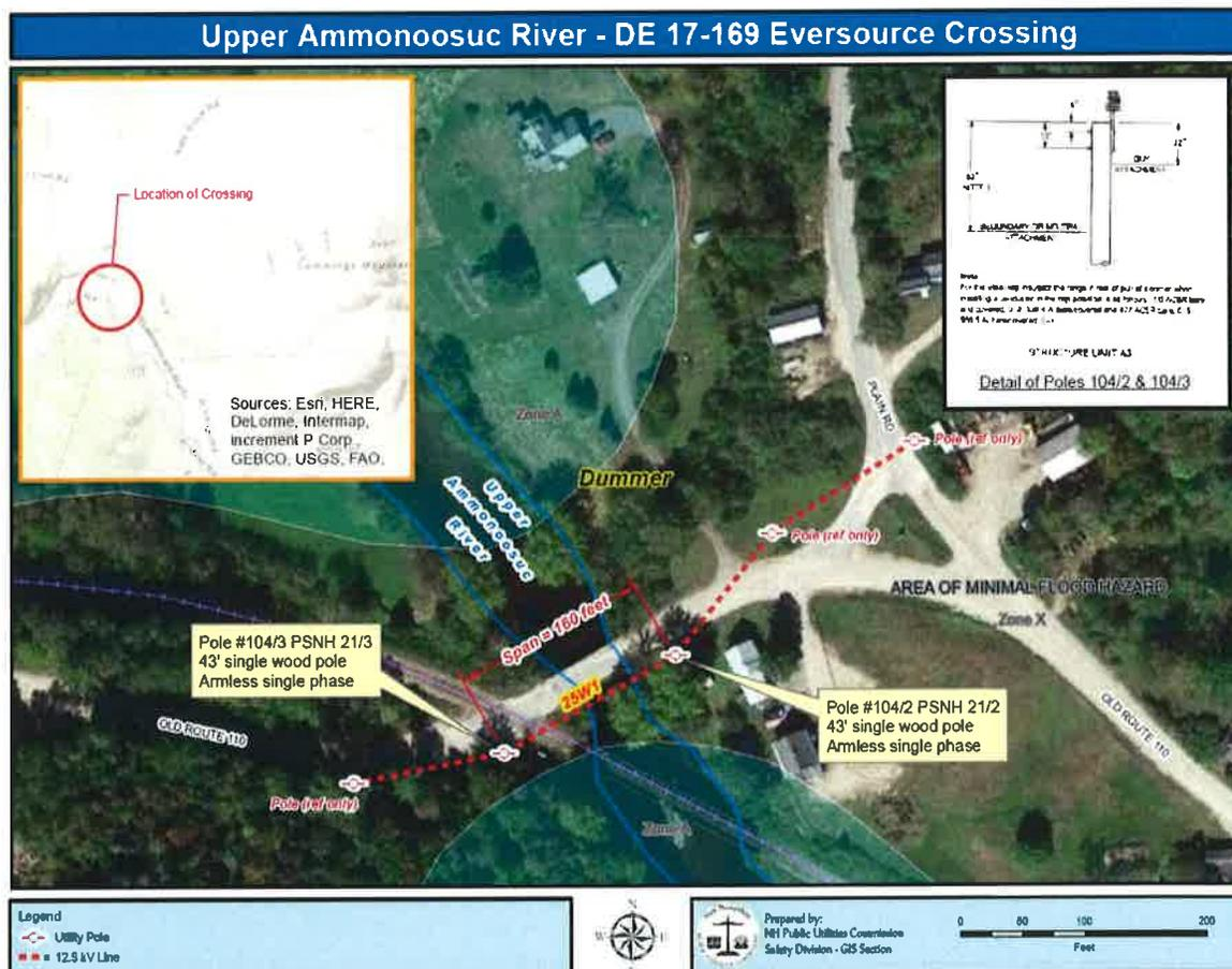
**Figure 1:** 7.2 kV, designated as the 25W1 Circuit, a span of approximately 160 feet, across the Upper Ammonoosuc River in Dummer, NH. The structures on the south side of the bridge are armless structures designated #21/3 and #21/2 to be constructed with a single class-2, 50 foot tall, CCA pole (embedded 7 feet). The span of the river is approximately 100 feet at the east and west banks, with the span from pole to pole 160 feet.
