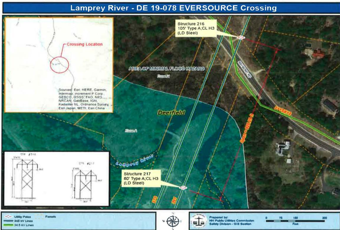
**Figure 1:** 345kV line, designated as the 391 Line, is a span of approximately 926.29 feet between structures # 216 and #217, across the Lamprey River in Deerfield, NH.
