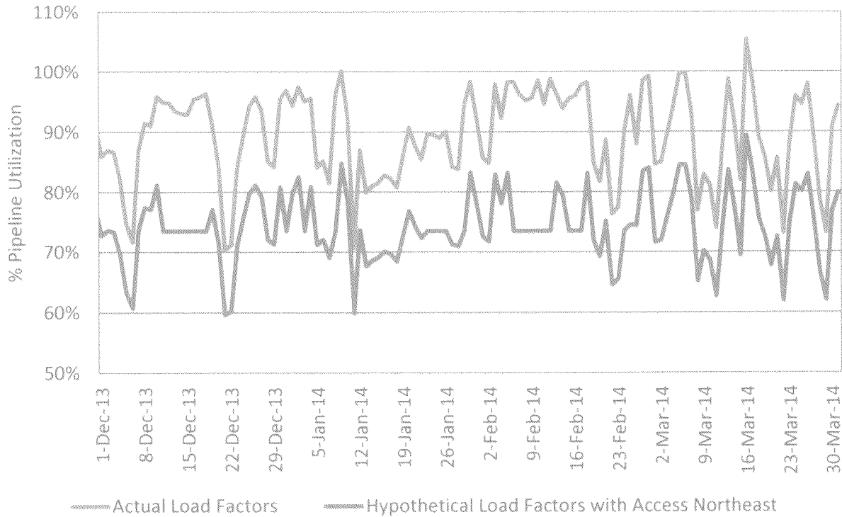
Exhibit 17: Actual Pipeline Load Factors and Hypothetical Reduced Load Factors with Access Northeast
