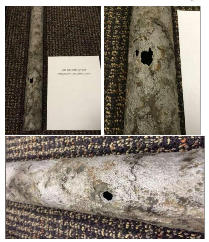
large holes with 100% wall loss on the exposed steel.
