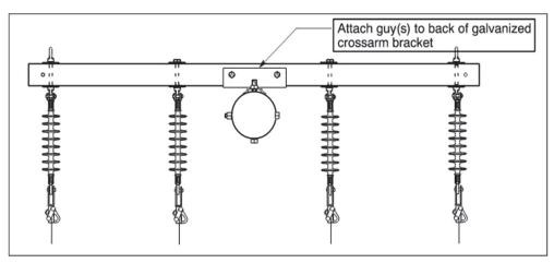
Figure 5-16. 27.6 kV Fiberglass Crossarm Construction, Three-Phase Dead-end Pole
