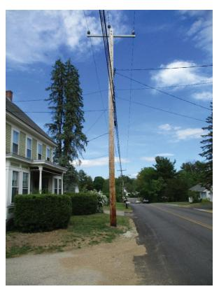
Figure 5-6. Example of Class 2 wood pole with fiberglass crossarm
