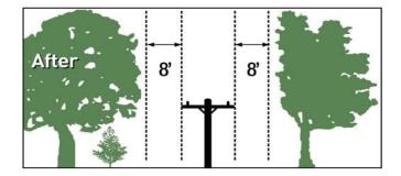
**Full-Width ROW Clearing:** ROW clearing allows an easement that has been encroached upon with vegetation to be fully cleared and restored to the full easement width from when the line was originally constructed. Once restored, future vegetation management will be performed with SMT.
