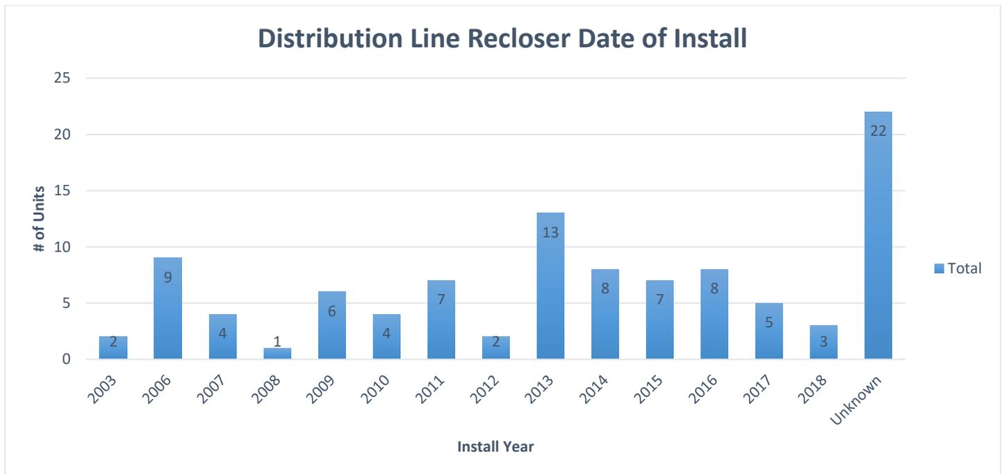
From a technology standpoint, the vast majority of the population is Cooper Power System products using either a Form 3, 3A, 4C, 5 or 6 control. The Form 3 and 3A controls are at the end of their service life. All new recloser installations will be Viper-S or ST using a Switzer SEL-651R control with remote status and control. All existing reclosers without communications will be evaluated for implementation of remote status and control capabilities.
