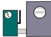
Meter socket, 480Y/277V, with unfused meter disconnect switch, cold sequence
