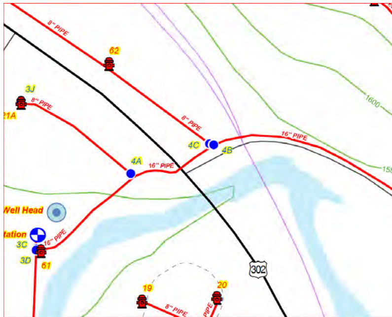
Figure 2-1 indicates an area in which excavation was performed near the 16-inch diameter water main between valves marked 4A and 4B but no markings by AWC were shown. Puc 800 rules require markings of any underground water mains within the tolerance zone or method of providing positive response that there are no such facilities within the tolerance zone. AWC did neither.
