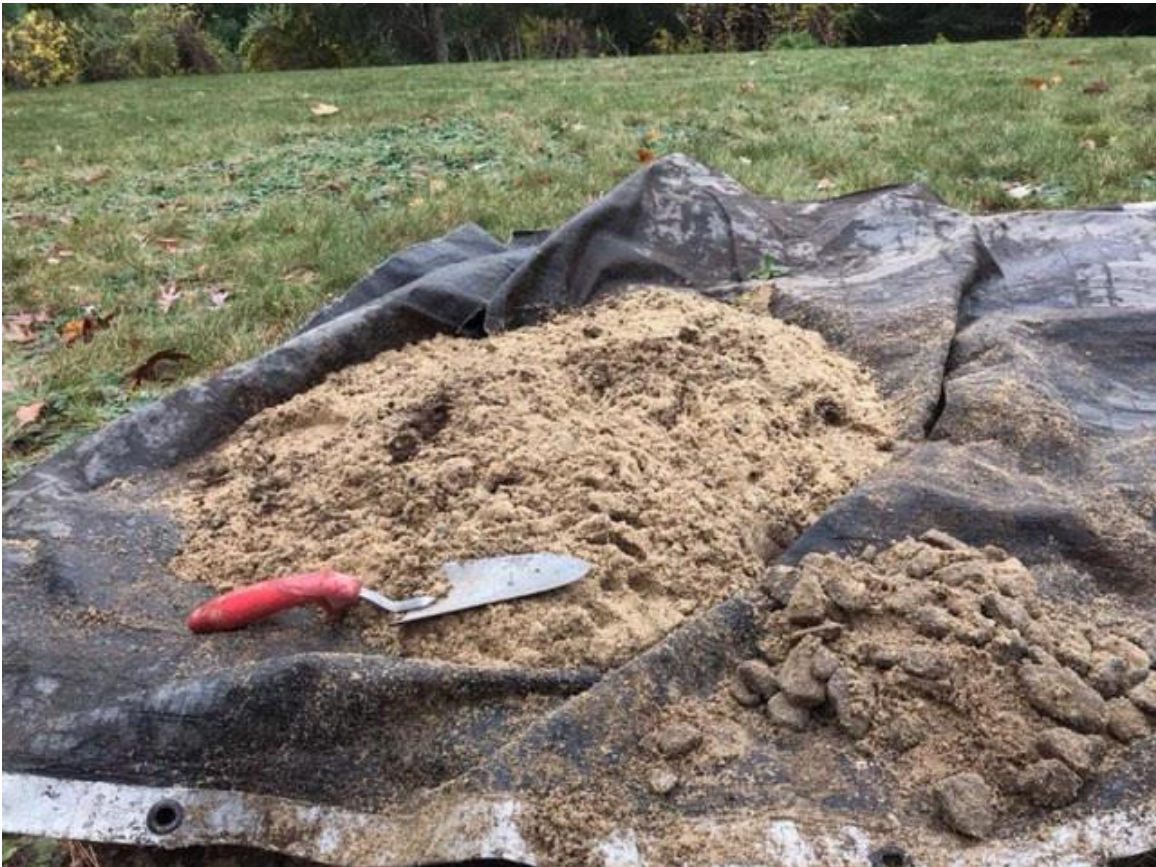
FIELD C – Observation hole #2 sand and stone
