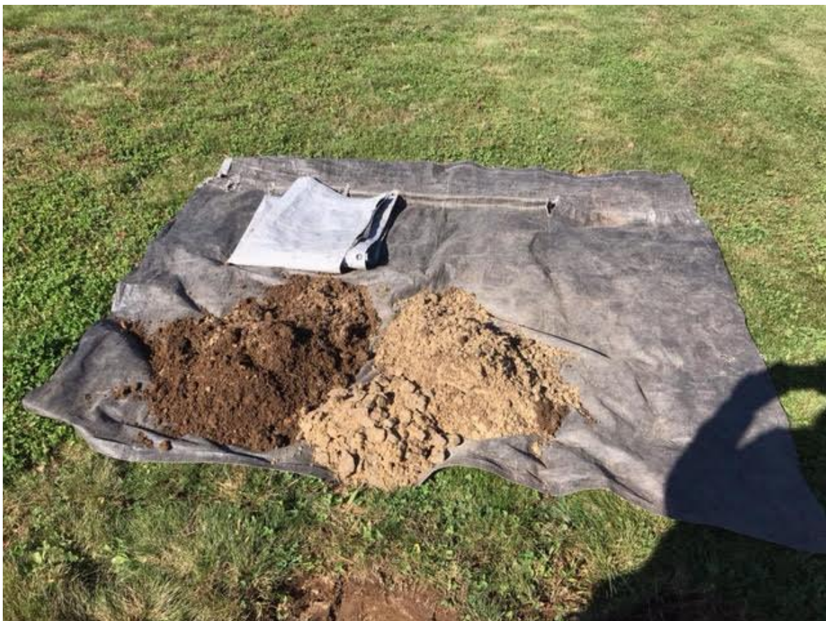
FIELD A – Observation hole #2 sand and stone
