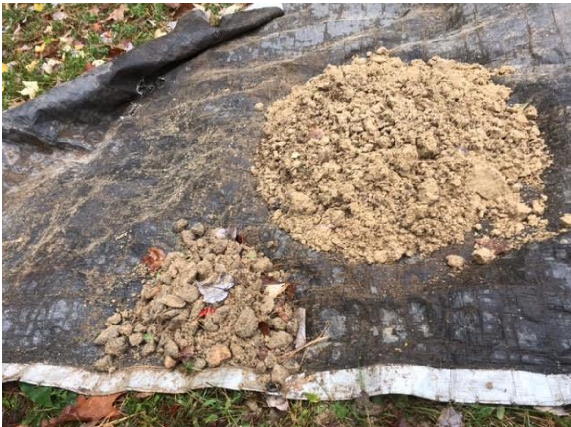
FIELD G – Observation hole #4 sand and stone
