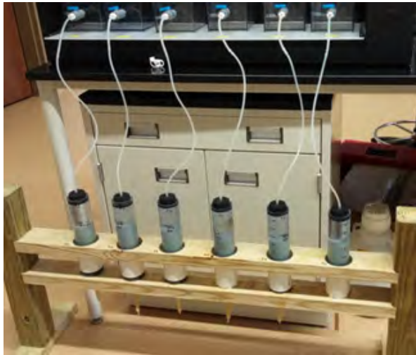
Media filtration-based bench scale jar testing apparatus developed by Stantec's Amir Alansari.
